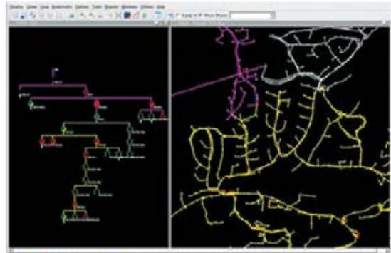
*Geo feeder display with schematic generator*
